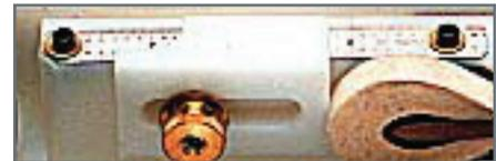
When drilling hammers that are less than 7/16" wide, you may have to loosen the Vice Knob to keep adequate pressure on the hammer.
