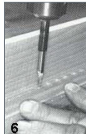
7. If you will be installing springs, place the mylar tape on the top of the damper tray, **being careful to index it so that the drillings will be directly over the drillings for the flange screws**. Renner USA has also provided a score line in the proper position for the underlever assist springs. With the mylar tape in the proper position, mark out with a prick punch the scale for the spring drillings.
