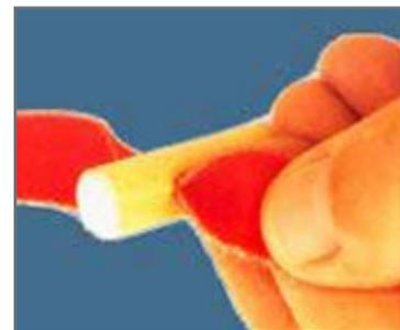
3. Bush the holes, applying a light coating of glue to the end of the cloth before pulling it into the hole. Trim the cloth leaving 1/4" protruding on one side of each bushed part.
