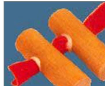
4. Before the glue has set, wet the bushings with rubbing alcohol and insert the pin, or drill or other rod of equal diameter. Push the pin in from the side that has the protruding cloth; this prevents the pin from forcing the bushing out of the hole. Put in a warm place to dry thoroughly.
