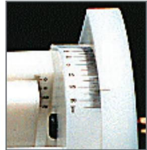
The rake angle is set by loosening the Locking Knob, pulling on the Spring Pin, and lining up the edge of the Rake Bar to the proper mark on the Rake Angle Gauge. The pin is set at 90° to make squaring up the rake for grands fast and easy. Rotate rake until it pops in place.
